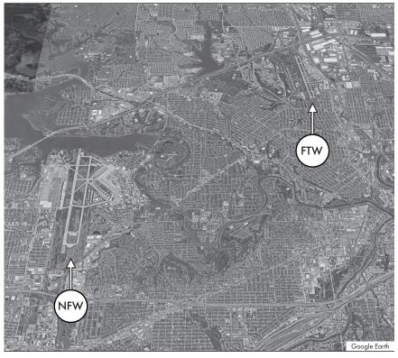
NFW is approximately 5.5 miles Southwest of FTW Airport and its RWY is 4500 ft. longer and 50 ft. wider than FTW RWY 16/34. Pilots confuse NFW RWY 18 with FTW RWY 16. Pilots confuse NFW RWY 36 with FTW RWY 34.
