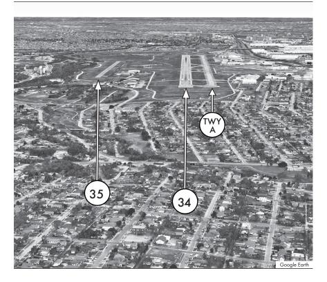
Pilots confuse RWY 35 for RWY 34. RWY 34 is over 3500 ft. longer, twice the width and over 1700 ft. closer than RWY 35. Pilots confuse TWY A for RWY 34.
