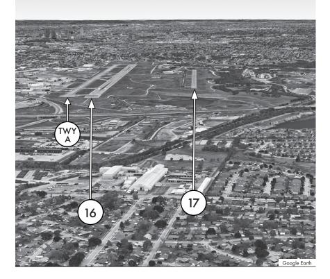
Pilots confuse RWY 17 for RWY 16. RWY 16 is over 3500 ft. longer, twice the width and over 1700 ft. closer than RWY 17. Pilots confuse TWY A for RWY 16.
