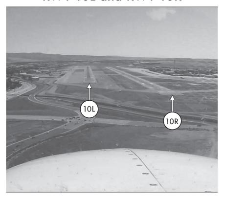
Use caution for closely aligned parallel runways with offset thresholds.
