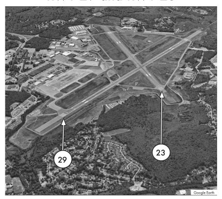
Pilots confuse RWY 23 for RWY 29 due to terrain features and/or proximity of runway thresholds.
