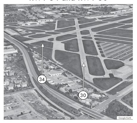
Use caution when circling East to land RWY 34 due to RWY 30 in close proximity. Ensure you are aligned with the correct runway and seek clarification from ATC if needed.
