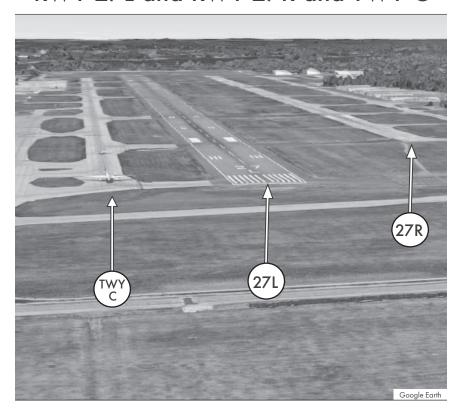
Off-set parallels. RWY 27R is 900 feet further down the approach than RWY 27L. Pilots sometimes confuse RWY 27L for RWY 27R, or TWY C for a runway.
