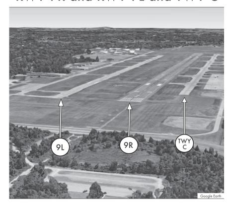
Closely spaced parallels. Pilots sometimes confuse the wider RWY 9R for RWY 9L, or TWY C for a runway.
