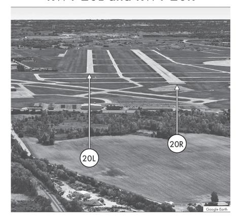
Off-set parallels. Pilots be aware that RWY 20L is 1120 feet farther down the approach than RWY 20R. Also, 20R is 50 feet wider than 20L.
